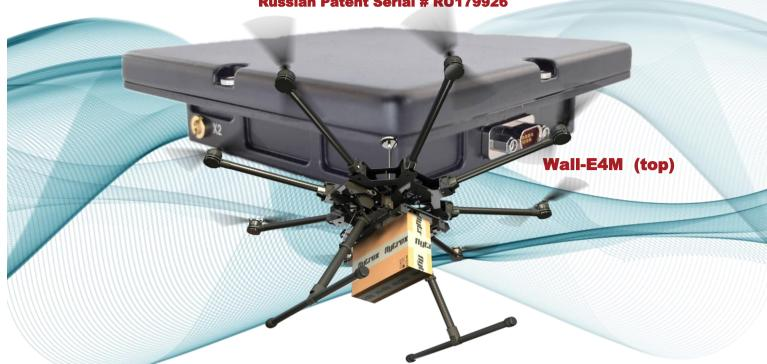
RIMCO JSC Wall-E4M is a 4-element GNSS Controlled Reception Pattern Antenna (CRPA) canmitigate/nullone interference or jamming signals in Global Navigation Satellite System (GNSS) bands offer higher protection against electronic warfare systems (EW) threats. Signal processing algorithms detect interference signals and amplitude and phase from each antenna element are adjusted in real-time to either to form a null in the direction of the interference source (null steering).
